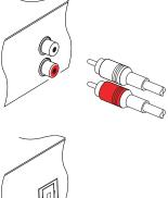
You will need to obtain an audio cable (RCA cable) to connect the audio connectors. Plug one end of the cable into the AUDIO L (white) and AUDIO R (red) sockets on the digital receiver, and the other end into the matching sockets on your television or audio system.
